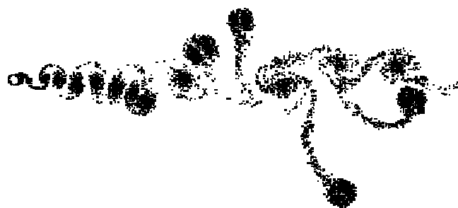
Figure 6. Discrete vortex particle positions for Re=1000 at \tau=50.00 using a hybrid diffusion velocity/random walk method.
