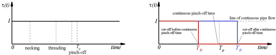
FIGURE 6. Comparison of (a) the continuous case indicating the characteristic drop formation stages of necking, threading and pinch-off with characteristic pinch-off timescale  $T_p$ , with (b) the discrete case showing flow discontinuity with characteristic timescale  $T_D$  shorter (red) and longer (blue) than the continuous timescale  $T_p$ .
