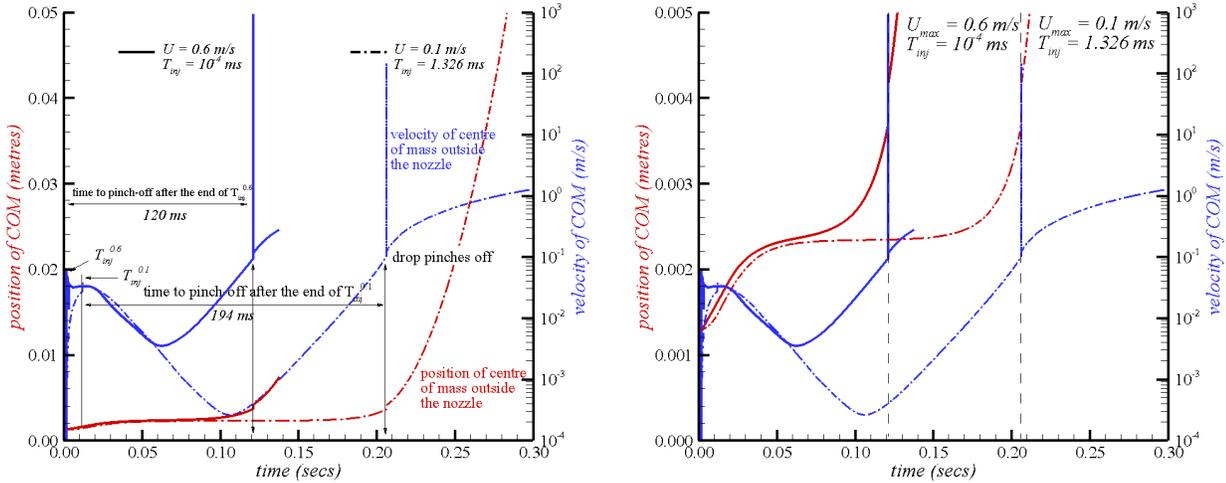
FIGURE 17. Plot showing (a) the change in the position and velocity of the centre-of-mass of the pendant drop with time and (b) a closeup of the region just before pinch-off
