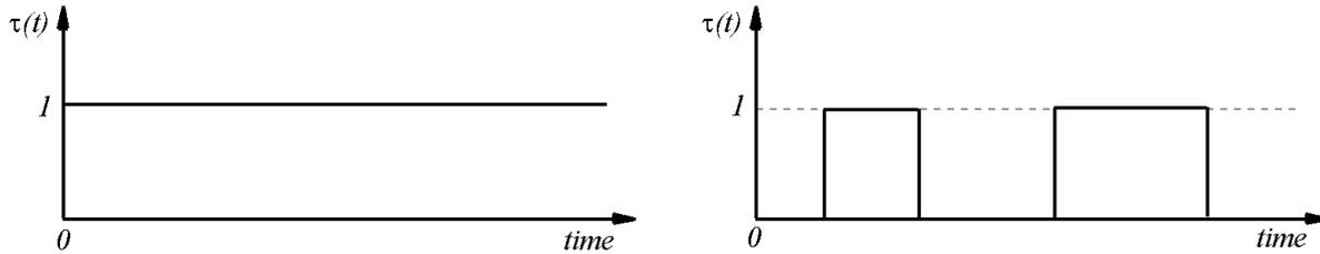
FIGURE 2. Plots of the time dependent part of the internal pipe flow  $\tau(t)$  for (a) a typical continuous process with a constant time dependent component and (b) a simple discrete process with a discontinuous time dependent component.
