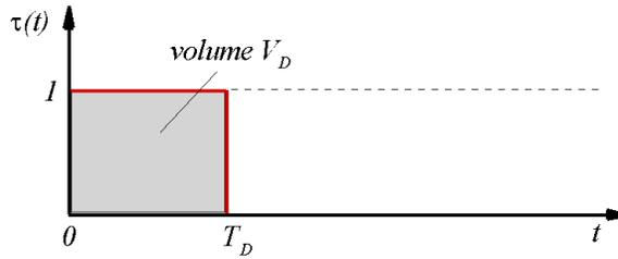
FIGURE 5. Diagram showing a typical step-wise time dependent component of discrete pipe flow axial velocity over a discrete time  $T_D$  and delivering an implied discrete volume  $V_D = \pi R^2 U T_D / 2$
