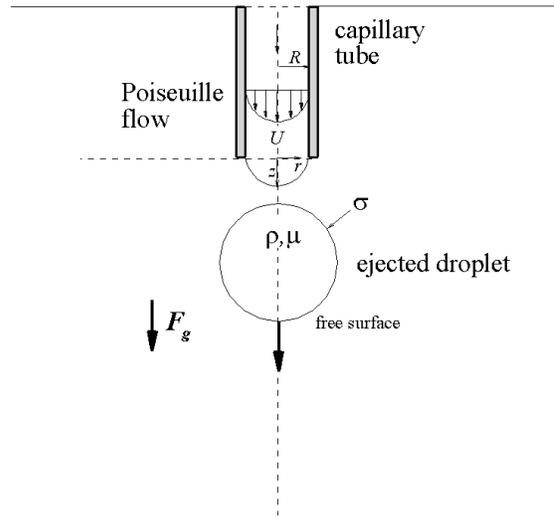
FIGURE 1. Drop ejection parameters and fluid dynamical scales.
