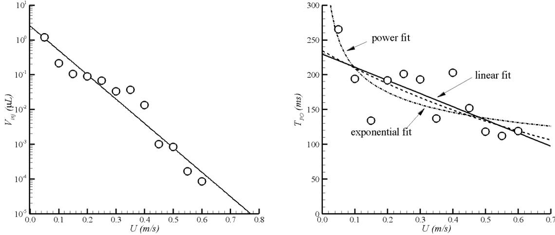
FIGURE 13. Plots of (a) critical ejection volume  $V_{crit}$  as a function of pipe flow velocity  $U$  for  $V_{pend} = 13 \mu\text{L}$  and (b) a graph showing the total time to pinch-off  $T_{PO}$  after the flow is turned off.
