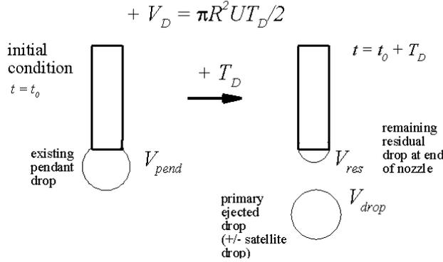
FIGURE 9. Diagrammatic process of drop ejection by adding a discrete volume  $V_D$  onto the existing pendant drop volume  $V_{pend}$  at  $t = t_0$  to eject a drop of volume  $V_{drop}$  after a time  $t = t_0 + T_D$ .
