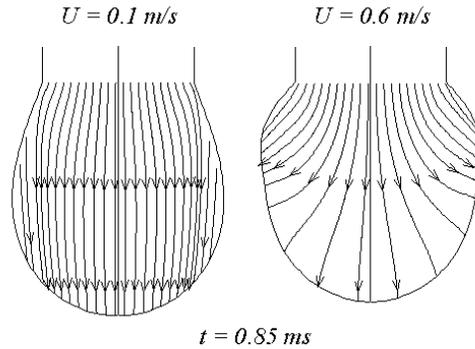
FIGURE 14. Streamline plots of the magnitude of velocity  $|\mathbf{u}|$  of drop formation at the capillary exit for (a)  $U = 0.1$  m/s (left) and (b)  $U = 0.6$  m/s (right) showing streamlines within the forming drop.
