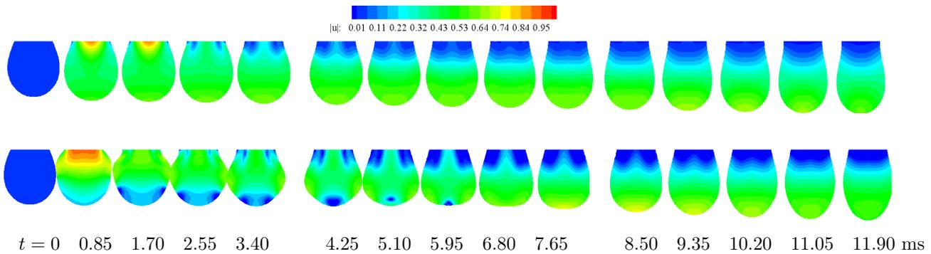
FIGURE 15. Contour plots of the magnitude of velocity  $|\mathbf{u}|$  of drop formation at the capillary exit for (a)  $U = 0.1$  m/s (top) and (b)  $U = 0.6$  m/s (bottom) at times after the flow is turned on. (N.B. all contour plots are shown in non-dimensional form as defined in Section 4, equations (6)-(11).)
