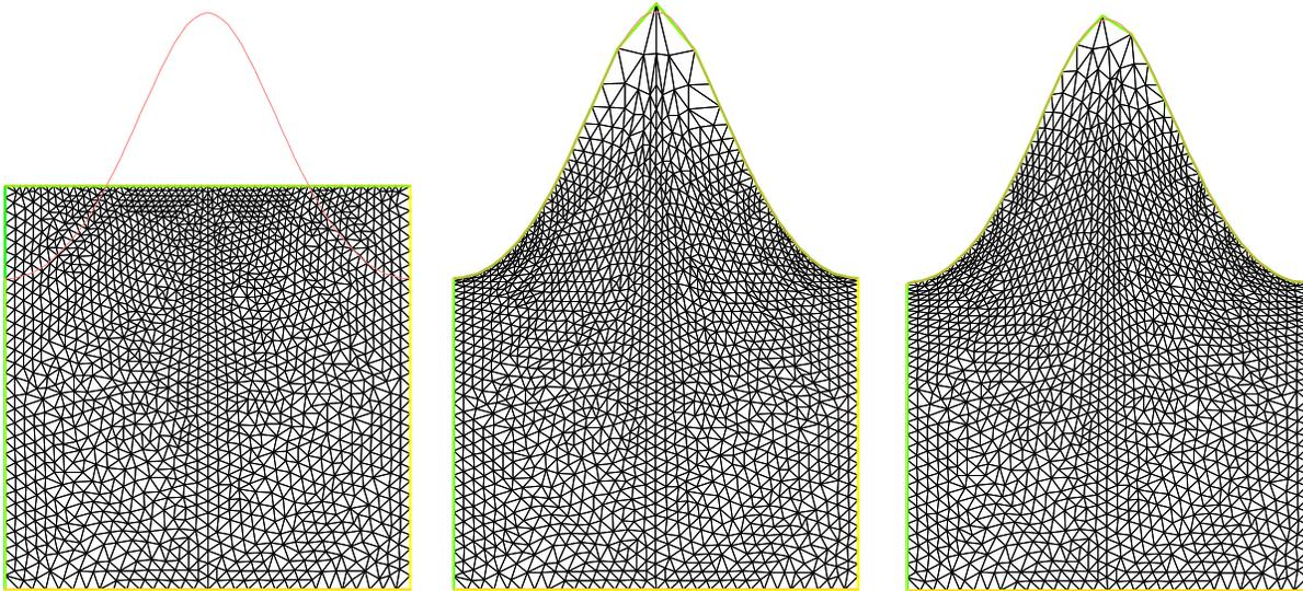
FIGURE 18. Left: reference mesh  $\mathcal{T}_{ref}$ ; Middle: deformed mesh  $\mathcal{T}_{map}$  using  $(\cdot, \cdot)_{elas,F}$ ; Right: deformed mesh  $\mathcal{T}_{map}$  using  $(\cdot, \cdot)_{elas,\kappa}$ .
