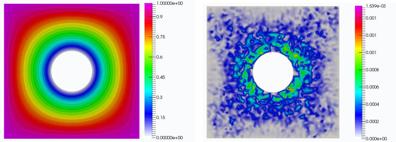
FIGURE 5. Left: solution  $\phi_{\text{map}}$ ; Right: relative error between  $\phi_h$  and  $I_h\phi_{\text{map}}$ .
