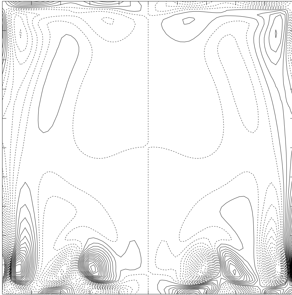
Figure 3: Contour plot of \omega_1 at the center plane \{x = \frac{1}{2}\} computed using second order 3D scheme. Parameters: Re = 3200, t = 15, CFL = \frac{\Delta t}{\Delta x} = 2.5, \Delta x = \frac{1}{64} .
